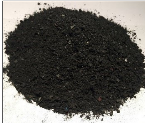
Production of "black mass" through mechanical process
